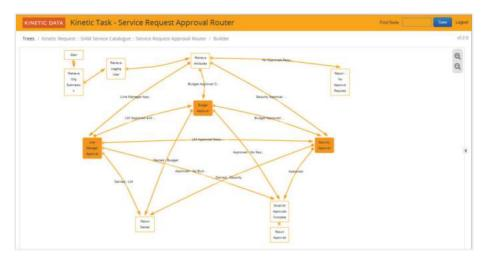
Mapping approval workflow using the Kinetic Task Drag+Drop Editor
